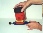
8. To change studs for Aviation or Auto filter, place in vise to disassemble stud and standoff or cutter wheel.
